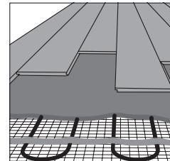
When installing BerryAlloc LVT on top of electric cables, a suitable levelling compound has to be used, on which BerryAlloc LVT can be installed, following our general installation instructions.
