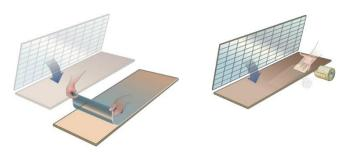
Apply BerryAlloc Adhesive on the existing wall (or on the backside of the panel) in strings formed as the letter "U". Let the strings cover 25-30 cm in vertical height and 5 cm in horizontal width, from top to bottom.
