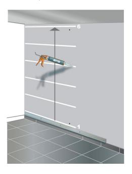
3b) Walls with max. deviation 12 mm per 2 m
