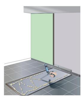
4) Re-position the W&W panel (w/adhesive). Put pressure on the panel and fasten the W&W panel to the wall with BerryAlloc screws, by using the pre-drilled holes in the locking profile.
