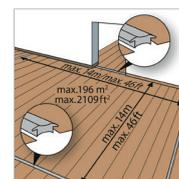
BerryAlloc laminate should be installed as floating flooring which means that the floor should be able to move:
